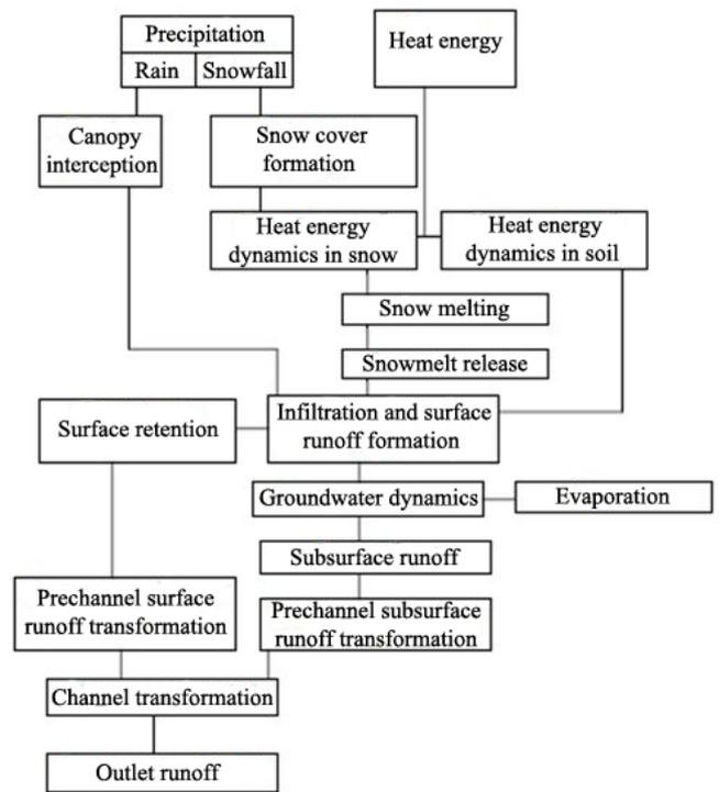
Figure 1. Diagram of the “Hydrograph” model.
