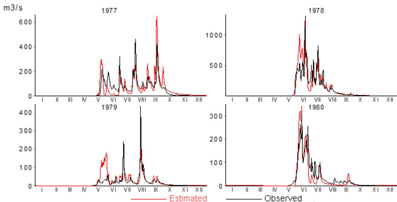
Figure 3. The estimated and observed runoff hydrographs in the upper reaches of the Kolyma basin (1977–1978: the Detrin River, the mouth of the Vakhanka River; 1979–1980: the Tenke River, 2.2 km from the mouth of the Nilkoba River).
