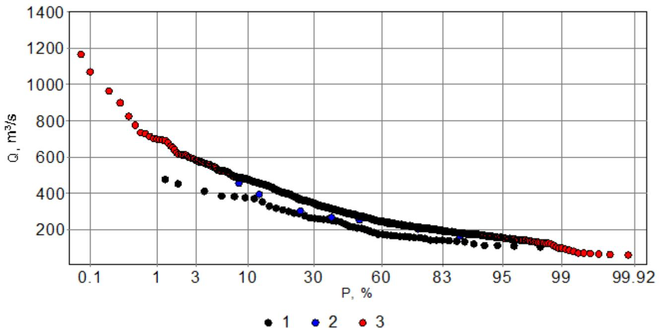
Figure 4. The curves of distribution of the estimated and the observed maximum water discharge ( $\text{m}^3/\text{s}$ ) in the Tenke River basin, 2.2 km from the mouth of the Nilkoba River (1, 2, 3 - see text).
